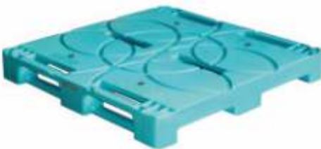
Model : AP1111SC Dimensions : 1100 (L) x 1100 (W) x 140 (H) mm. approx. Load Bearing : Uniformly Distributed Load : Static : 3600 kg. • Dynamic : 1200 kg. • Racking : 600 kg. Should be handled with Forklift or Pallet truck only.
