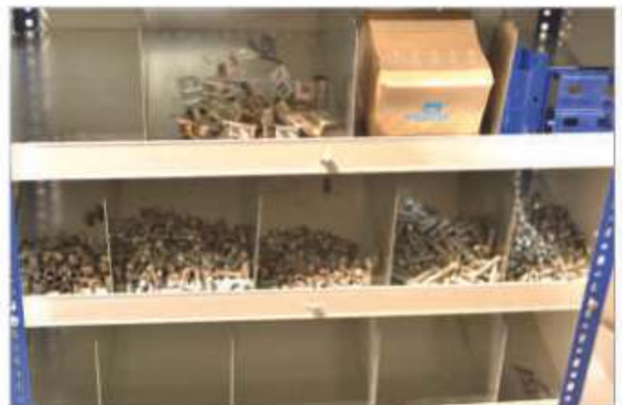
Store. Stop spilling over...!! : Front stopper strips hold back the contents of the storage partitions from spilling over.
