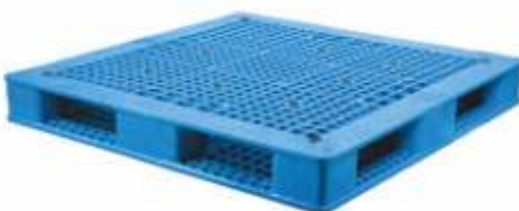
Model : DP1212 Dimensions : 1200 (L) x 1200 (W) x 150 (H) mm. approx. Load Bearing : Uniformly Distributed Load : Static : 6000 kg. • Dynamic : 1500 kg. • Racking : 1000 - 1500 kg. Should be handled with Forklift only.
