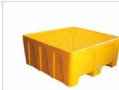
Model : RMPC525L3RSPIIL • Dimensions : 1300 (L) x 1300 (B) x 575 (H) mm. Pallet with lid • Stacking : Ground +2 • Sump capacity : 525 liters
