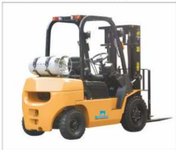
Model : NK20LPG / NK30 LPG • Capacity upto (kg) : 3000 Lift Height upto (mm.) : 6000 Mast : 2 Stage / 2 Stage FFL / 3 Stage FFL
