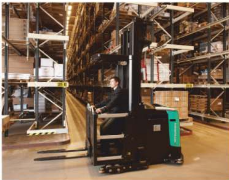
High Level Order Picker Model : OPBH10N/10NH Capacity (kg) : 1000
